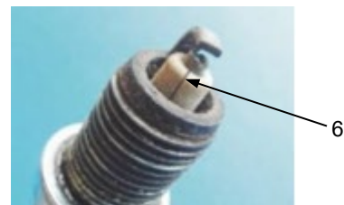
Figure 3: Spark Plug with crack (6) in porcelain Insulator
